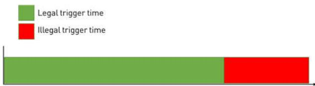
A window watchdogs feature a time-window, in which it expects to be triggered. Only if it is triggered within the window, it is properly reset. If it is triggered outside of the window, it will report an error. Window watchdogs therefore not only allow checking if user-code is executed within a maximum time, but also introduce a minimum time. With window watchdogs, it becomes possible to monitor if software is executed within defined timing constraints.
